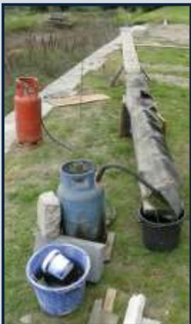
inserted into one end of the inner tube which had been cut across to create a tube, (somewhat curved but beggars can't be choosers!). This was then propped up at an angle and connected to the steamer by means of a length of old washing machine hose.
