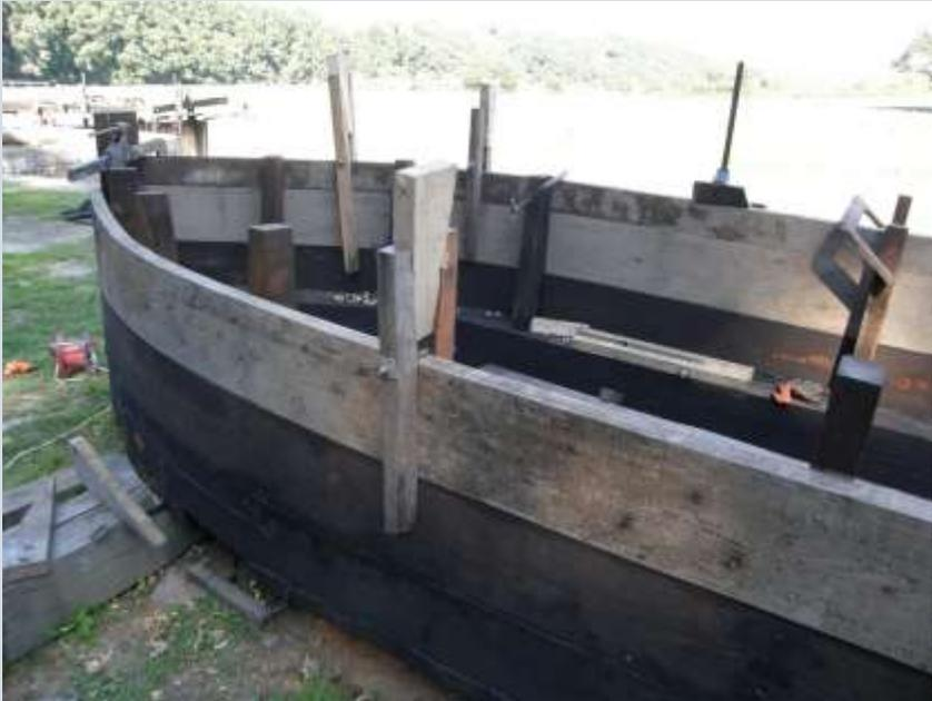
This picture shows one of the 'clothes peg' style clamps, made by Barry, specifically for holding the cladding while it was being bent to shape and fixed in place.
